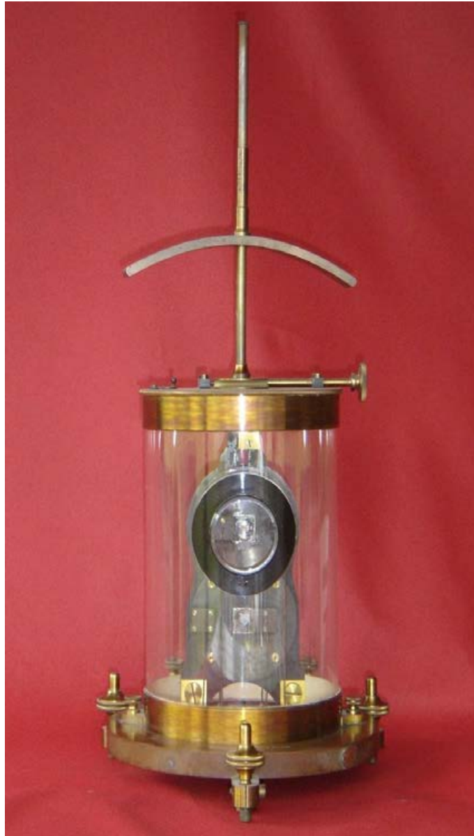
My high-grade four coil differential astatic Thomson mirror galvanometer, made by Louis Breguet
